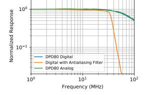
Figure 2: Frequency response of the DPD80. <sup>3</sup>
