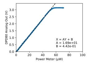
Figure 5: Analog output power calibration. High gain mode.  $^4$
