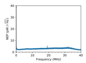
Figure 1: Digital noise floor at 10 Hz BW. High gain mode.  $^{\rm 2}$
