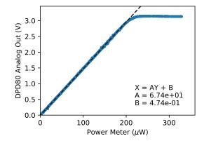
Figure 6: Analog output calibration. Low gain mode.
