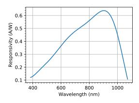
Figure 7: Spectral sensitivity
