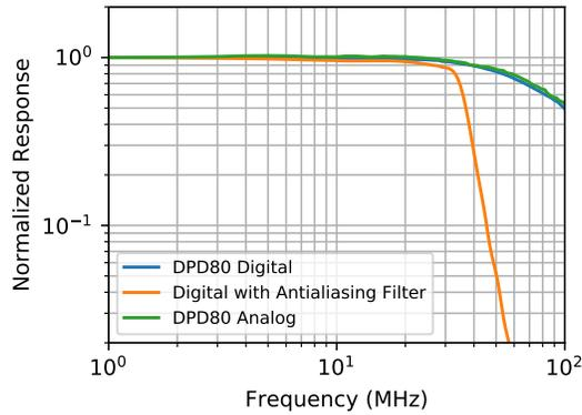
Figure 5: Frequency response of the DPD80. <sup>2</sup>
