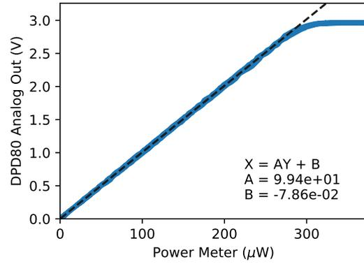
Figure 9: Analog output power calibration. Low gain mode.<sup>3</sup>
