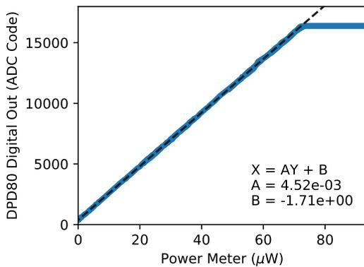
Figure 6: Digital ADC power calibration. High gain mode.
