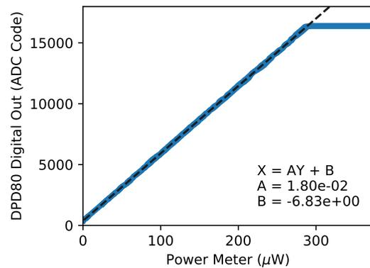
Figure 7: Digital ADC power calibration. Low gain mode.
