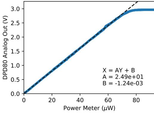
Figure 8: Analog output power calibration. High gain mode.<sup>3</sup>
