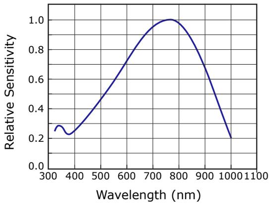
Figure 10: Spectral sensitivity
