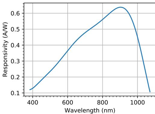
Figure 7: Spectral sensitivity
