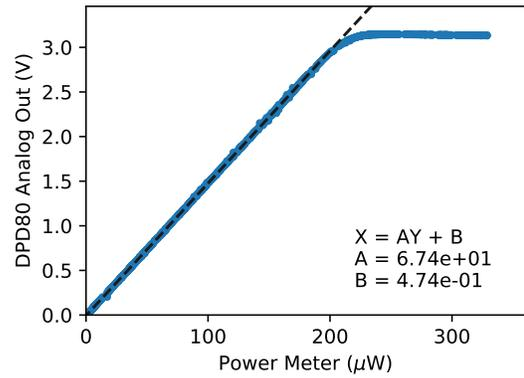
Figure 6: Analog output calibration. Low gain mode. <sup>4</sup>
