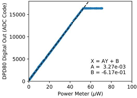
Figure 3: Digital ADC power calibration. High gain mode.
