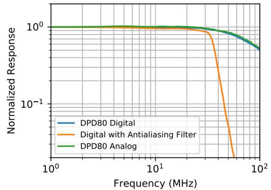
Figure 2: Frequency response of the DPD80. <sup>3</sup>
