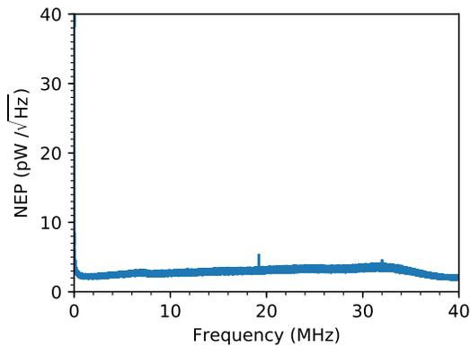
Figure 1: Digital noise floor at 10 Hz BW. High gain mode. <sup>2</sup>
