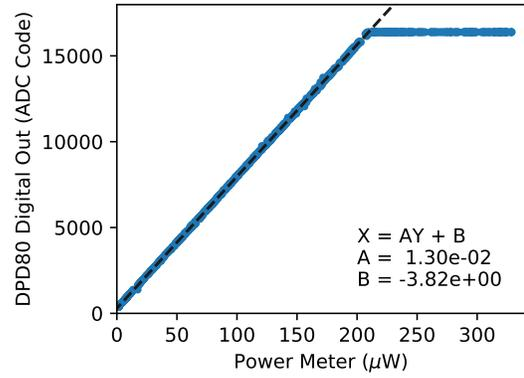
Figure 4: Digital ADC power calibration. Low gain mode.
